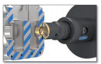
Roller burnishing an end face of a gear housing with type RP
