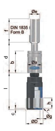
Burnishing heads are replaceable within the diameter range. By request, the tools can be equipped with selffeeding capability (recommended only for machines with manual feed (e.g. box column drilling machines)).
