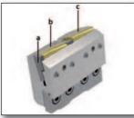
Skiving knife (a. Insert seats, b. finish cutter, c. pre-cutter)
